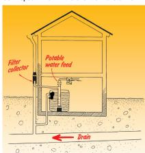
and torrential rainfall 50 % of the water is filtered and transferred to the storage tank. Excess rainwater is led directly to the drain or to infiltration.
