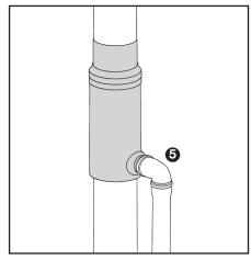
6 Connect the outlet connectin to the storage tank with 50 mm plastic pipe or steel pipe with a rubber gasket. To facilitate the rapid outflow of water from the filter, we recommend the use of a downward facing elbow on this outlet.
