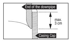
It is important to match the filter size with the correct pipe diameter. The top cap of the filter is designed to be a dose fit on the pipe to ensure that water flow is directed over the surface of the filter element.
