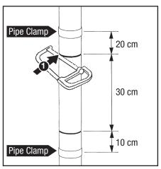
• Remove a 30 cm section of the rainwater downpipe at the desired installation height. Clean up the saw cut ends of the pipe with a halfround file.
