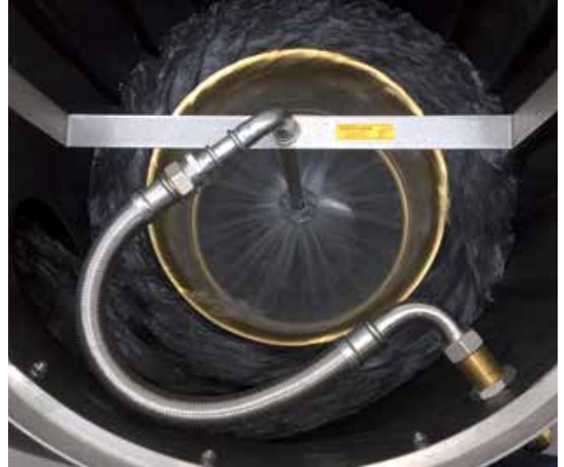
Cleaning nozzle for Vortex Finefilter WFF 300
