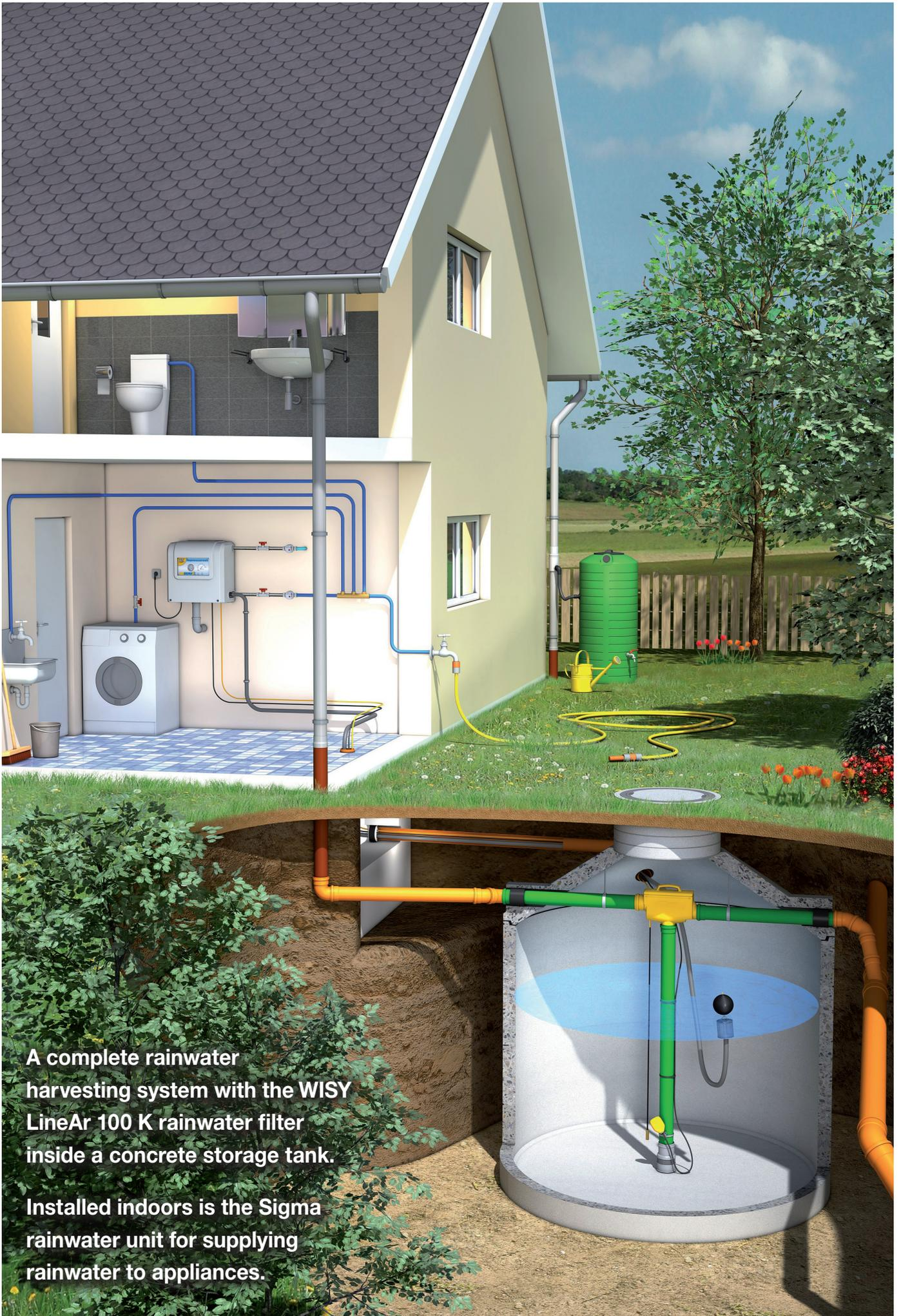
A complete rainwater harvesting system with the WISY LineAr 100 K rainwater filter inside a concrete storage tank.
