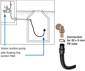
Suction hoses in precut lengths of between 0.75 m and 3 m, or supplied by the metre
