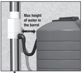
Integrated security overflow: the upper end of the outflow connection has to be levelled on the desired height of the maximum water level of the barrel. Thus the excess rainwater will automatically be diverted to the infiltration or drain.
