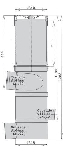
Outlet for dirt and rinsing water to the sewer or to the drainage system DN 150
