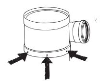
Now insert the screws back into the predrilled holes and tighten. Then connect up the rainwater inlet tube and the filtered water outlet tube.
