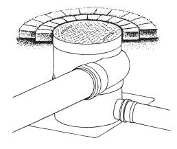
After these tubes have been connected, backfill all around the WFF 300 unit
