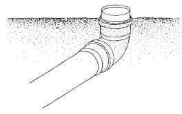
Fill and compact the hole around the storm drain pipe with sand, level out the sand surface. The short section of alignment tube should now be visible above the sand surface.
