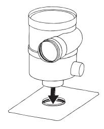
Once the plate is positioned, remove the alignment tube. Now place the WFF 300 housing into the open collar of the elbow and make sure that the surface pressure on the WFF 300 body is fully absorbed by the baseplate.
